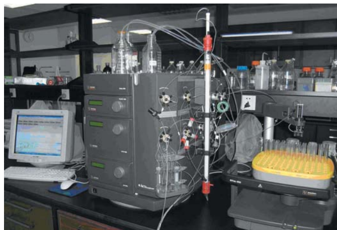
Figure 4 ÄKTA Explorer 100 with 3D kit for parallel purification of His 6 -tagged proteins.
