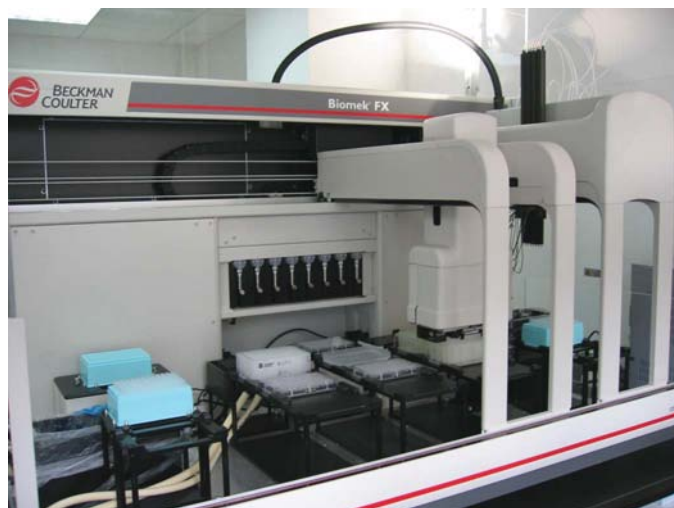
Figure 2 A multi-purpose liquid handler based on the Beckman Coulter Biomek FX automation system. It has been used for PCR, different kinds of DNA purification, ligation, expression checking, small-scale protein expression and some initial crystallization screening.
